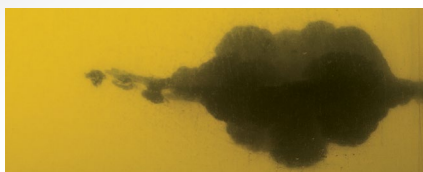
A17 17 HMR (949CC) shot into bare ballistics gel at 100 yards; 6 inches penetration.
