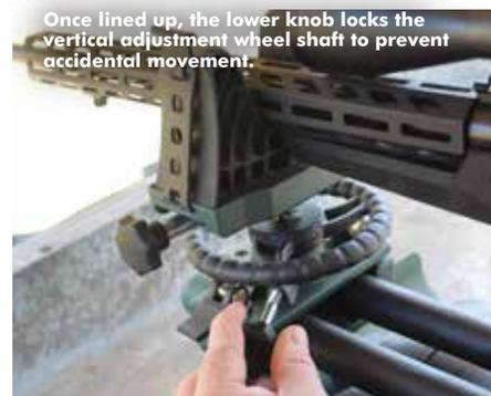
Once lined up, the lower knob locks the vertical adjustment wheel shaft to prevent accidental movement.
